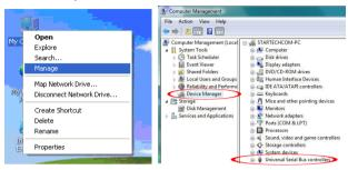
In the Device Manager, under the Universal Serial Bus Controllers category, you should see the new entries for the USB 3.0 controller card.
